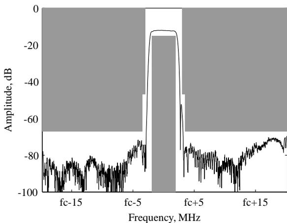
Figure 21: Response of a tapered SPUDT IF filter on Langa-site for a 3G basestation.
