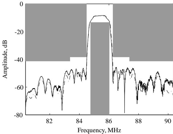
Figure 2: Frequency response of a dual track RSPUDT. Both theory (---) and experiment (—) are shown.
