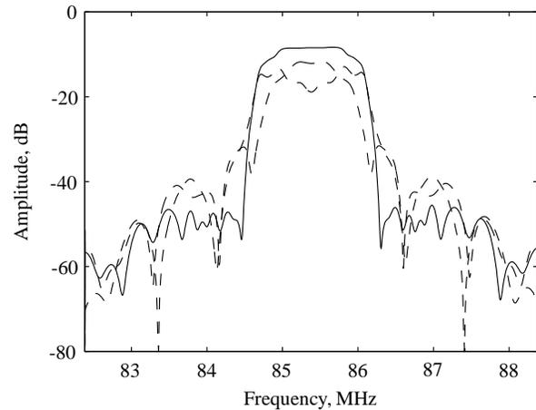
Figure 6: 900 MHz band CDMA IF filter (—). The frequency response of each track is shown dashed (---).
