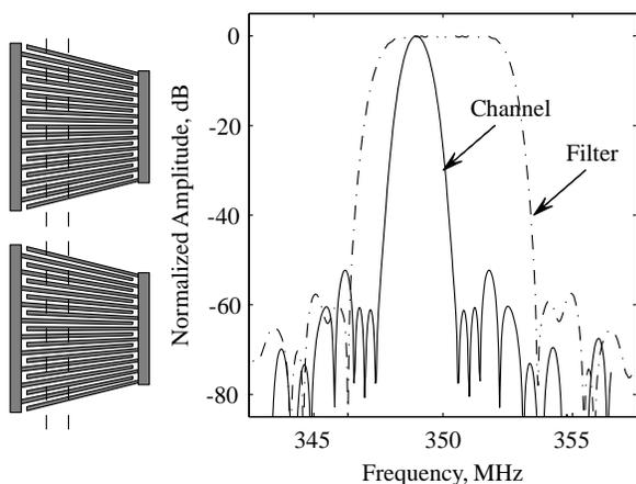
Figure 16: Tapered transducer filter (—) showing a single narrow channel (---).
