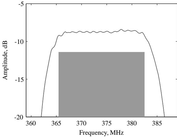
Figure 19: Passband response for the tapered SPUDT WLAN IF filter.
