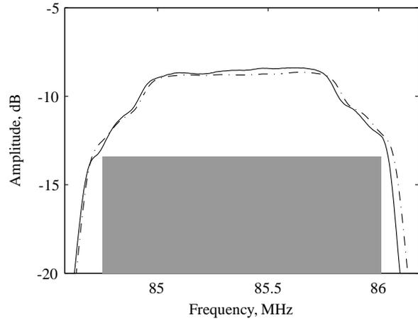
Figure 3: Passband response of a dual track RSPUDT. Both theory (---) and experiment (—) are shown.
