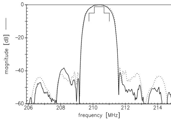
Figure 11: Measured (—) and predicted (- · -) frequency response of a recursive Z-path 1900 MHz CDMA IF filter.
