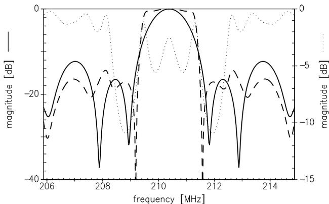
Figure 13:  $P_{23}$  of the input transducer with (—) and without reflectivity (- -).  $P_{21}$  (···) is also shown, and illustrates the resonances present in this transducer.
