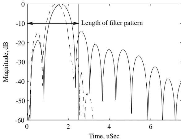
Figure 5: Impulse response for the dual track RSPUDT with (—) and without (---) reflectivity. The total length of the filter pattern on the die is noted.
