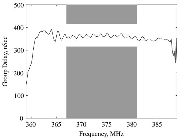
Figure 20: Group delay for the tapered SPUDT WLAN IF filter.
