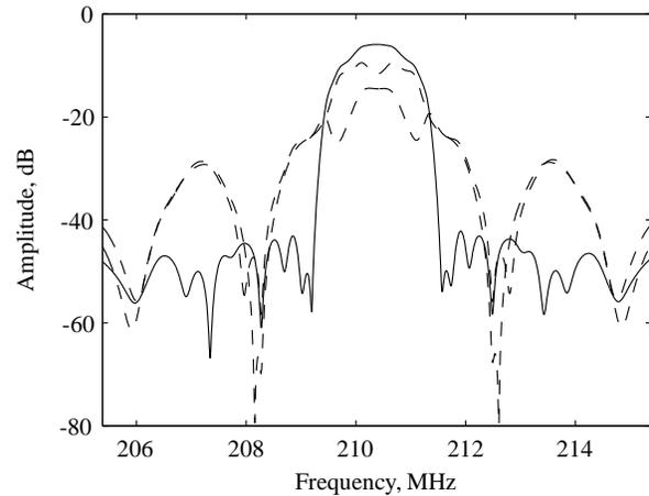
Figure 7: 1900 MHz band CDMA IF filter (—). The frequency response of each track as shown dashed (---).
