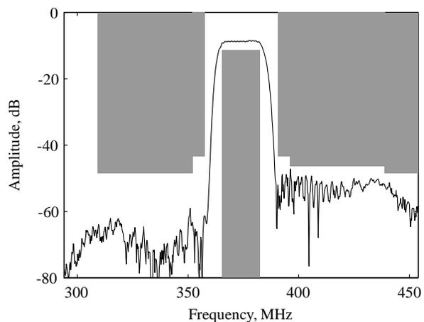
Figure 18: Frequency response for the tapered SPUDT WLAN IF filter.
