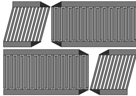
Figure 10: Schematic of a recursive Z-path IF filter.
