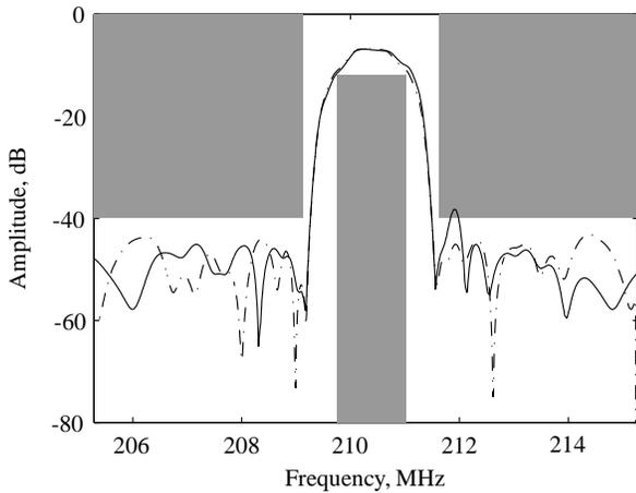
Figure 8: The effects of the local velocity variations are illustrated. The solid curve (—) represents a device with no correction for these velocity changes. The dash-dot curve (- · -) represents the measured response for a filter with correction for local the velocity changes.
