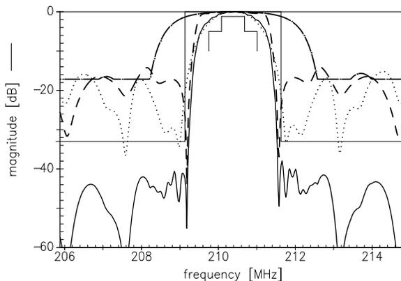
Figure 14: The overall frequency response of a recursive Z-path is comprised of the input transducer (- -), output transducer (···), and the included reflectors (- · -) which fold the propagation path.
