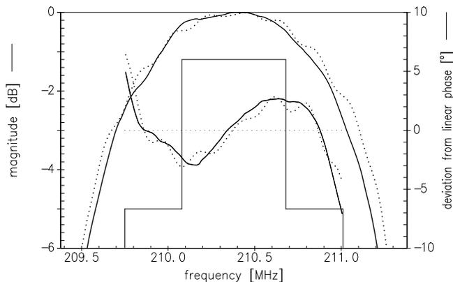
Figure 12: Measured (—) and predicted (···) passband response of a recursive Z-path 1900 MHz CDMA IF filter.
