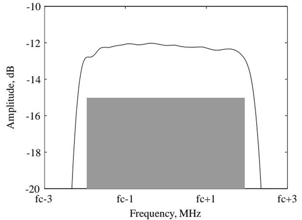
Figure 22: Passband of a tapered SPUDT IF filter on Langa-site for a 3G basestation.
