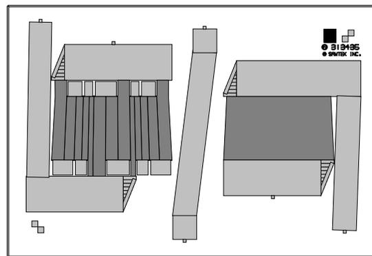
Figure 17: Simplified schematic of the WLAN tapered SPUDT IF filter. Block weighting is applied to the left transducer and withdrawal weighting to the right transducer.
