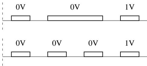
Figure 9: DART with and without reflection. Local changes in the transducer structure results in local changes in the SAW velocity.
