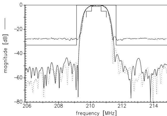
Figure 15: The frequency response of a filter without feed through cancellation is illustrated with (· · ·) and without (- · -) time gating. The 3rd response (-) is that of a filter with feed through cancellation.
