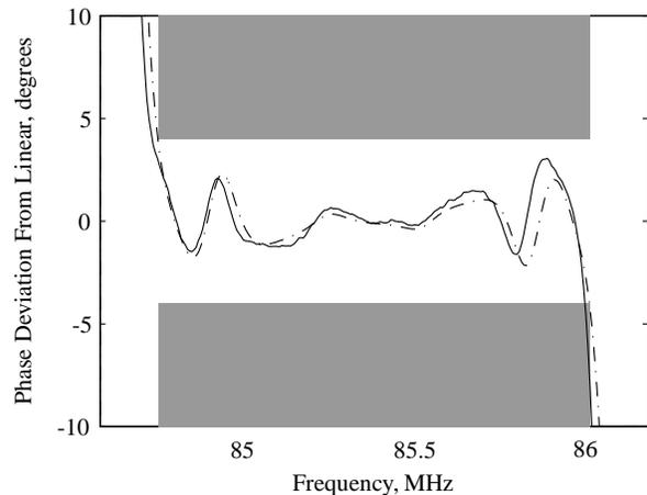
Figure 4: Phase deviation from linear of a dual track RSPUDT. Both theory (---) and experiment (—) are shown.
