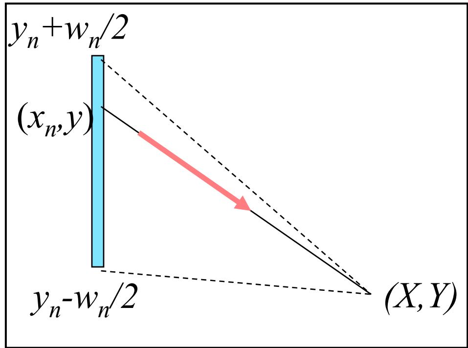
$$\phi(X, Y) = A \sum_{n=1}^N \int_{y_n - w_n/2}^{y_n + w_n/2} G(X - x_n, Y - y) dy$$
