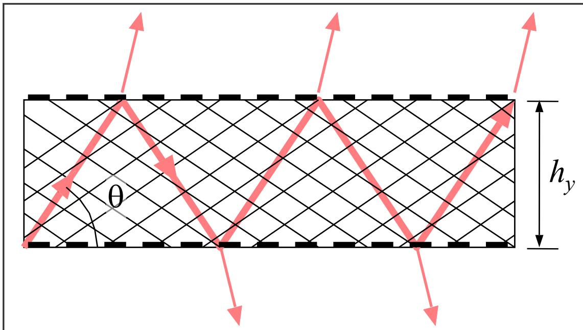
*When Reflection Coefficient at Surfaces is Large, Pseudo Mode Propagates with Energy Leakage to Outside*
